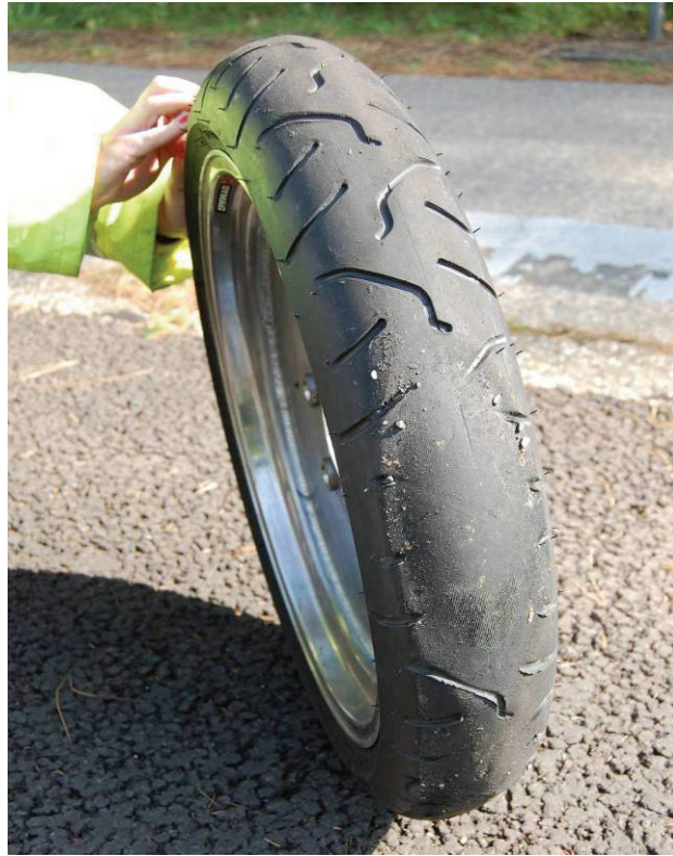
Figure 14: Tyre BT014 after completion of dry tests on HRA
