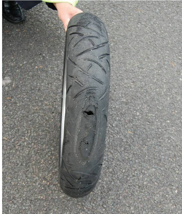
Figure 16: Tyre BT021 after completion of dry tests on HRA
