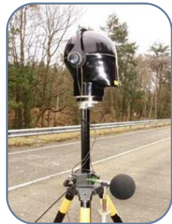
Figure 3.1: Set-up for binaural audio recording
