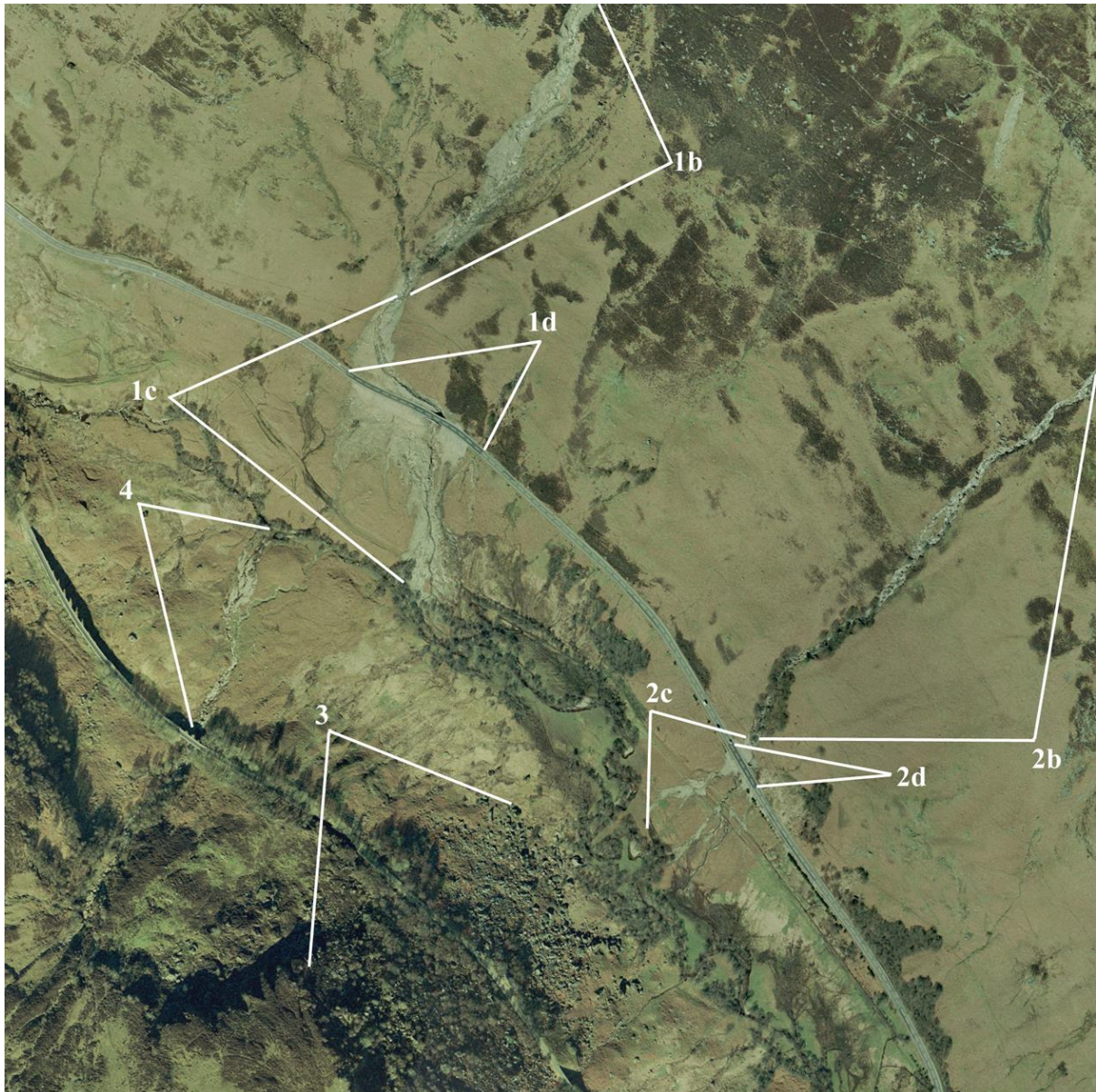
Figure 7. Aerial photograph showing the northerly (N) and southerly (S) debris flows that occurred in Glen Ogle in August 2004 with key features marked. The photograph represents a 1km by 1km square; north is to the top and the marked features are as for Figure 1, the south-west corner is located at National Grid Reference NN 570 260, or 2570 7260. (From Winter et al., 2009.)
