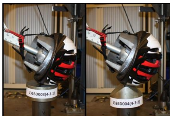
Figure 1: Wire guided linear headform drop test set-up for the impacting the right temporal region on flat and kerbstone anvils
