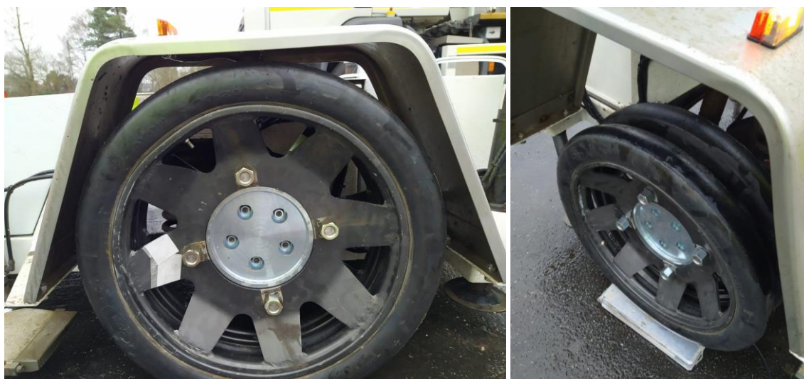
Figure 5-3 SCRIM tyres installed on the PFT
