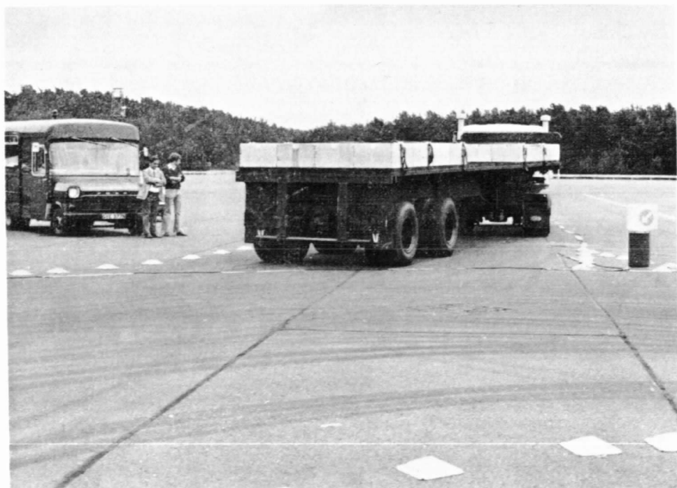
Plate 4 Fully loaded 32 ton GVW articulated combination 15.2m long completing a left turn
