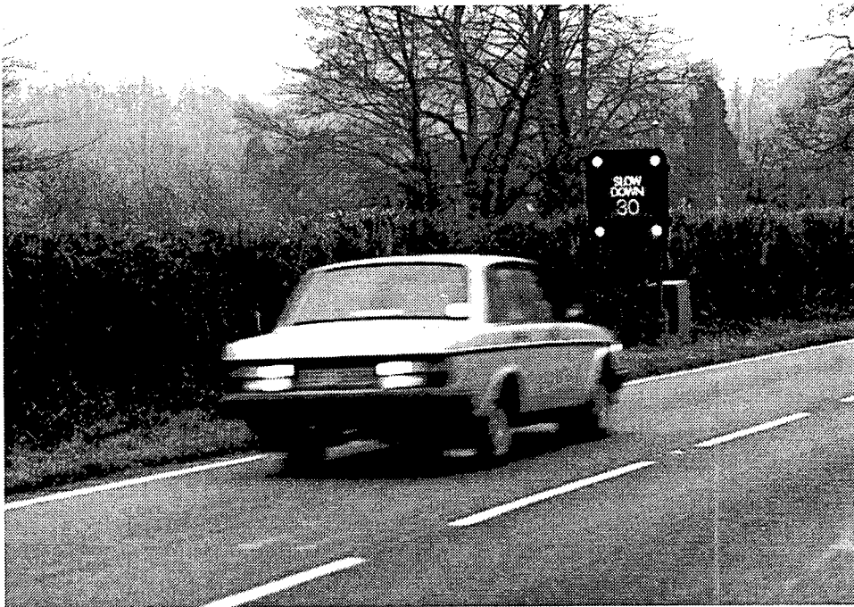
Example of a vehicle activated speed limit reminder sign (note flashing lights)
