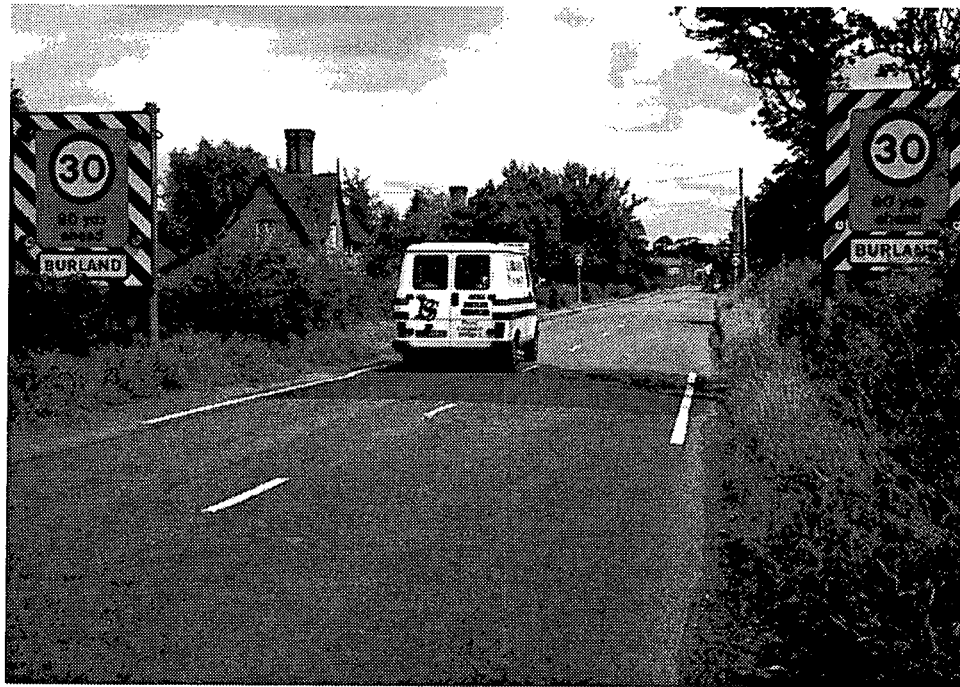
Fig 4 Enhanced sign at site 1, Burland. (note flashing lights, lower lit in photo)
