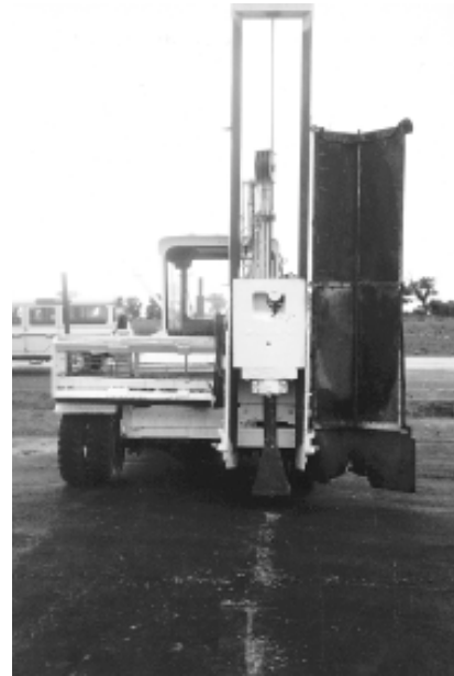
Plate 12 Arrows breaker - view of drop weight
