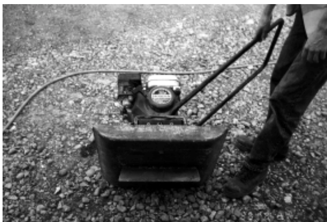
Plate 1 Vibrating plate equipment
