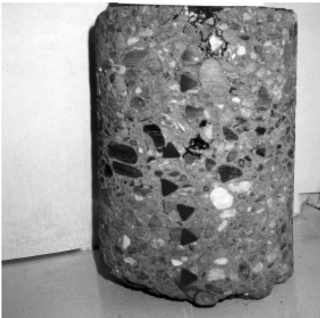
Plate 16 CBM core of crack formed using vibrating plate
