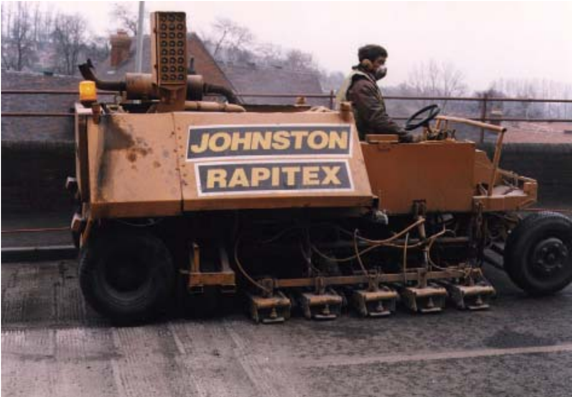
Photograph 14 Johnston Rapitex Durogrip machine
