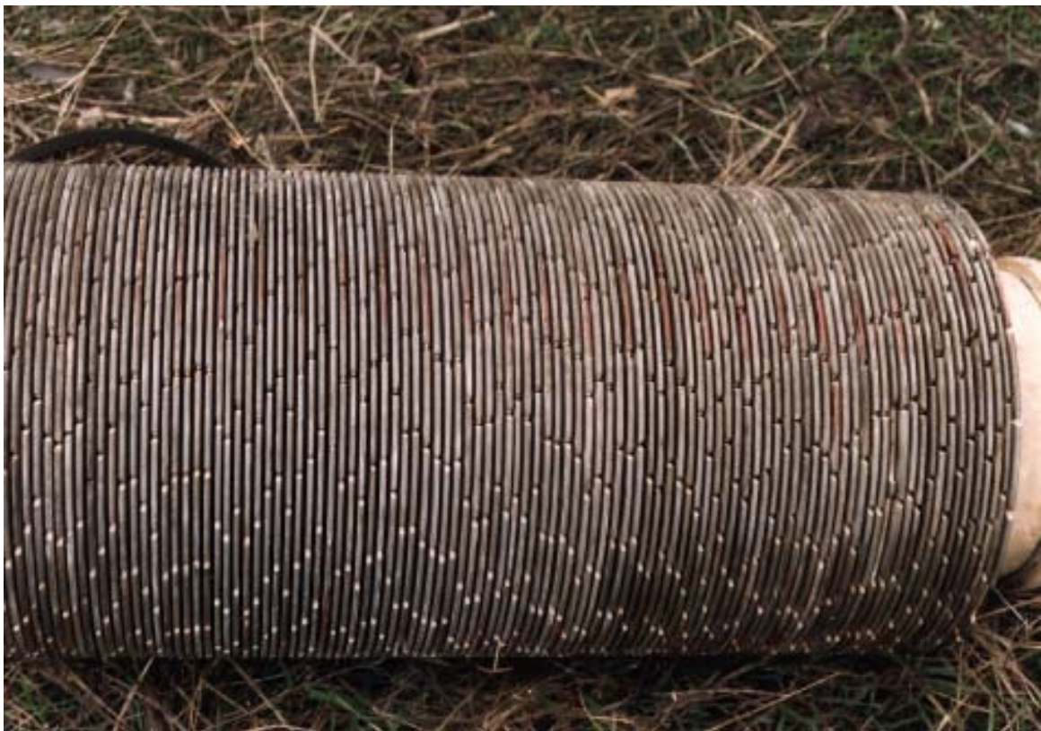
Photograph 6 Corduroy blades on Holemater machine
