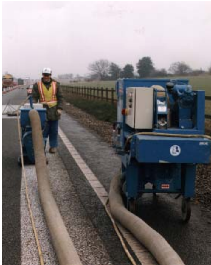
Photograph 3 France Grenaille shot-blasting machine
