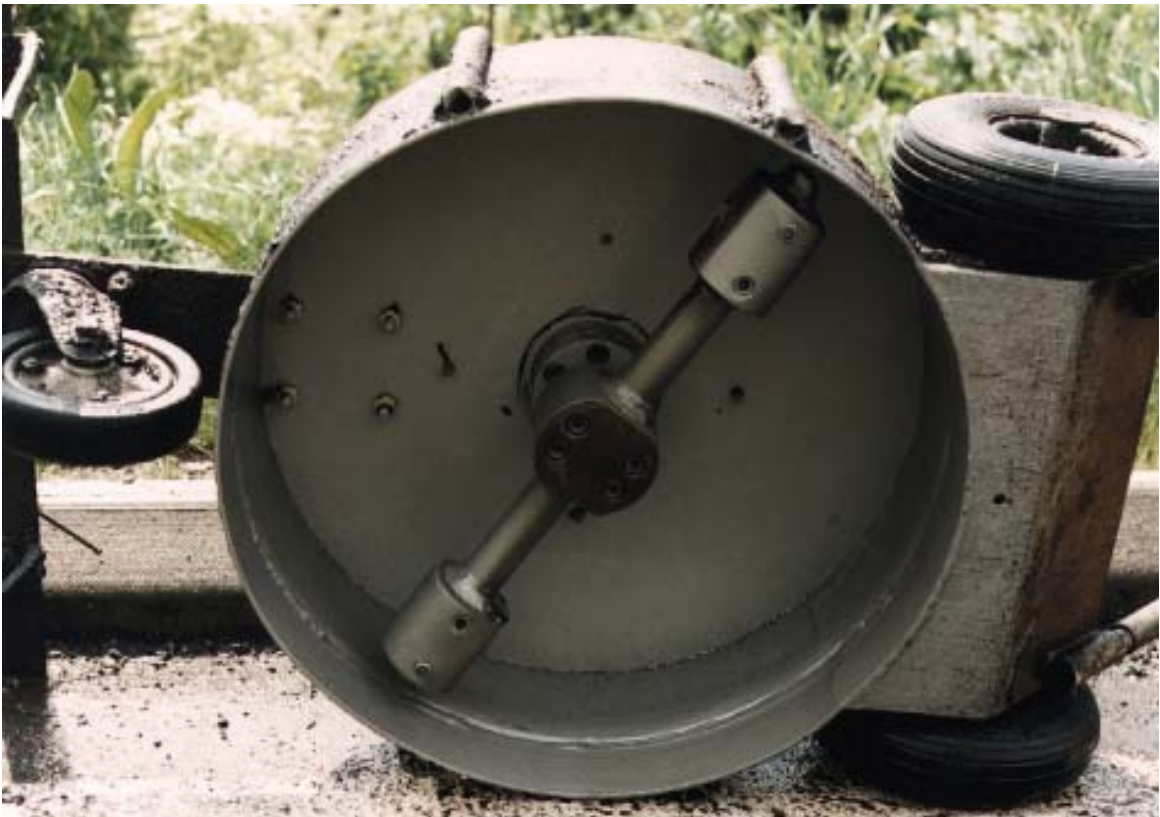
Photograph 18 Rotor bar and water jets on Watertex machine
