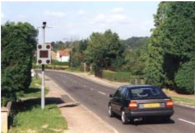
Figure 5 30mph fibre-optic speed limit sign, Longwater Lane
