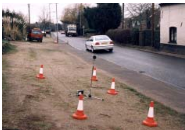
Figure A2 Arrangement for Statistical Pass-By measurements in West End (photograph taken during Before measurements)
