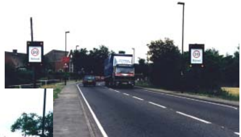
Variable message signing showing 20mph speed limit during school arrival and leaving periods (conventional 'school' sign at other times)
