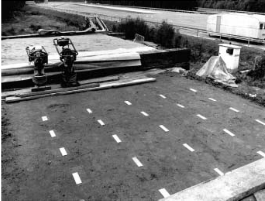
Figure 3 View of the embankment for the corrosion experiment at the Laboratory showing the arrangement of coupons and the compaction plant used
