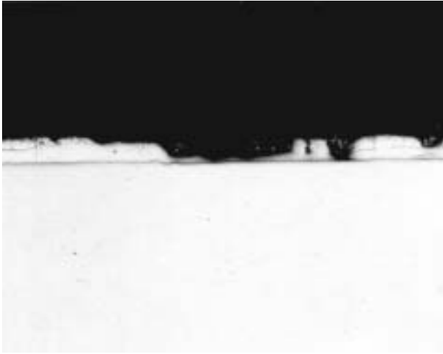
a Micrograph showing partial loss of galvanising (x100)
