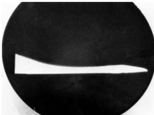
Figure 7 Profile of a particularly heavily corroded section of an aluminium alloy coupon recovered from the corrosion experiment at the Laboratory in 1990
