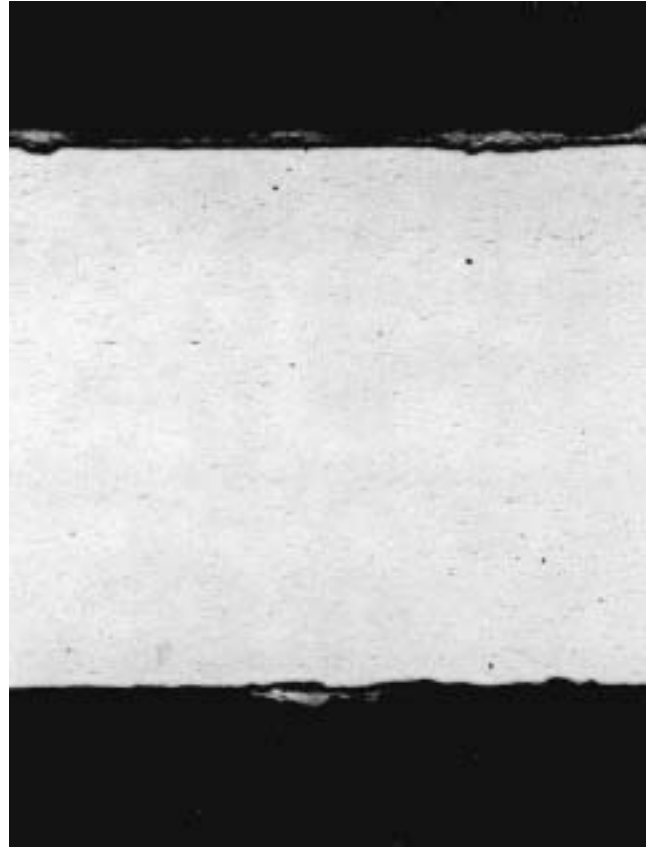
a Micrograph showing loss of galvanising (x20)
