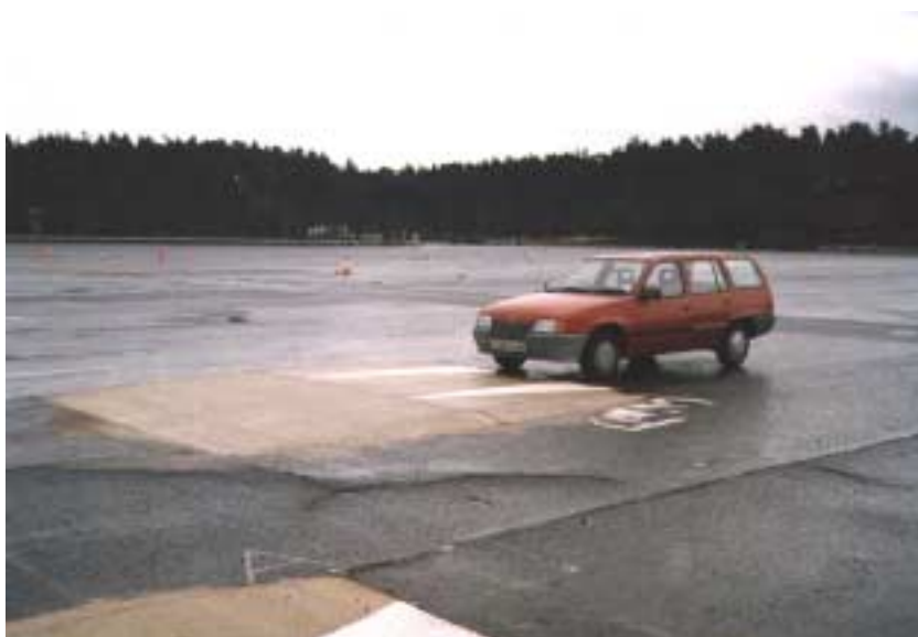
Plate 3 Profile P3, round-top hump, 5.0m long
