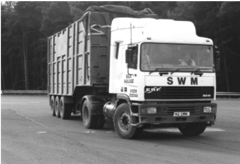
Plate 20 38 tonne ERF EC10 tractor and tri-axle trailer, steel suspension
