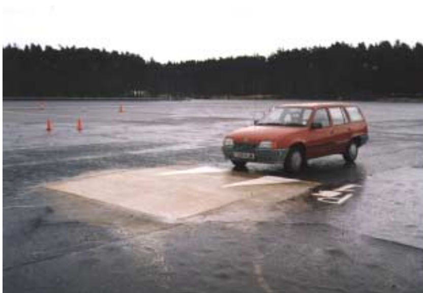
Plate 1 Profile P1, sinusoidal hump, 3.7m long
