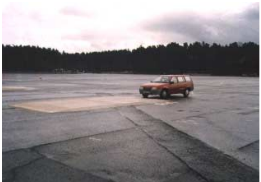
Plate 5 Profile P5, flat-top hump with straight ramps
