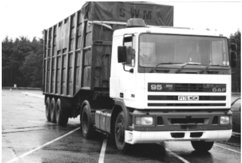
Plate 21 38 tonne Leyland DAF 95 tractor and tri-axle trailer, air suspension
