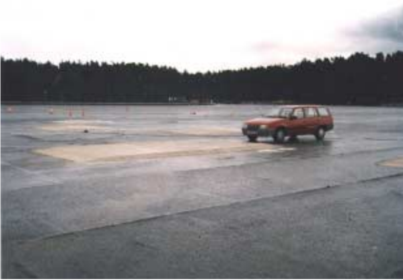
Plate 4 Profile P4, flat-top hump with sinusoidal ramps
