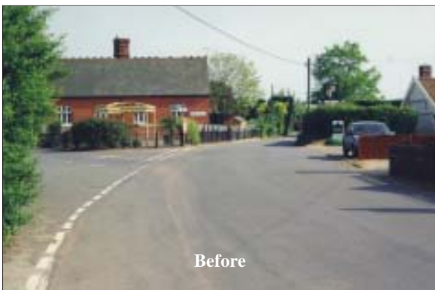
Figure 45 As Figure 44, showing the horizontal deflection feature viewed from the opposite direction, and the school. The Street continues round to the left, whereas Mill Road continues as the main road straight ahead. The surfacing was intended to reduce speeds of left-turning traffic but appears to have been cut across as illustrated by the tyre marks in the right-hand picture
