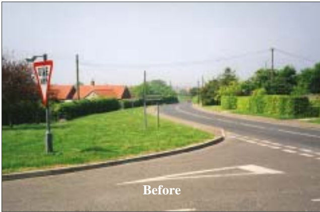
Figure 19 Blakeney: 1200mm illuminated 'give way' sign and 'Saxlingham' direction sign replaced by 600mm reflective 'give way' sign and road nameplate, junction of A149 with Saxlingham Road (looking west)
