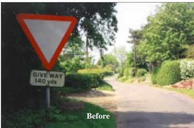
Figure 18 Blakeney: 1200mm advance 'give way' sign (left) replaced by 600mm sign, Saxlingham Road approaching A149
