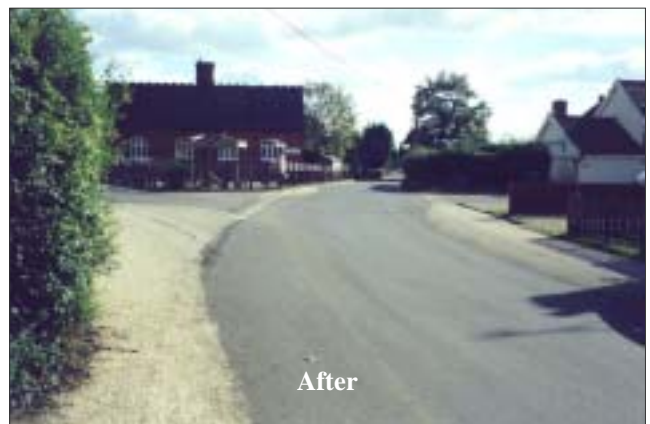
Figure 45 As Figure 44, showing the horizontal deflection feature viewed from the opposite direction, and the school. The Street continues round to the left, whereas Mill Road continues as the main road straight ahead. The surfacing was intended to reduce speeds of left-turning traffic but appears to have been cut across as illustrated by the tyre marks in the right-hand picture
