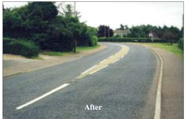
Figure 20 Blakeney: Overrunnable median strip of imprinted material to constrain speeds, at/near junction with Saxlingham Road (looking east)
