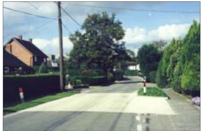
Figure 43 Kerbed and grassed build-out and light coloured surfacing on Mill road south-east of the village centre (looking north-west). Residents' parking bay also shown. Left-hand picture shows view before scheme intallation
