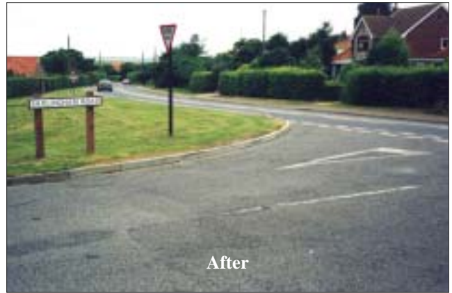
Figure 19 Blakeney: 1200mm illuminated 'give way' sign and 'Saxlingham' direction sign replaced by 600mm reflective 'give way' sign and road nameplate, junction of A149 with Saxlingham Road (looking west)
