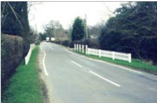
Figure 9 Russ Hill – fencing and hatched edge markings inside the gateway
