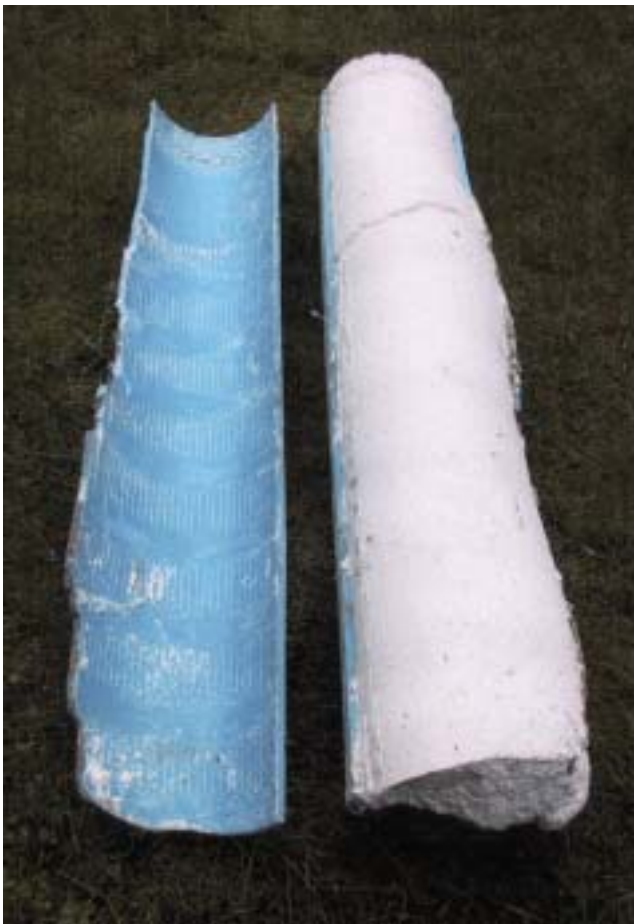
Plate B2 Removal of lime pile from its casing
