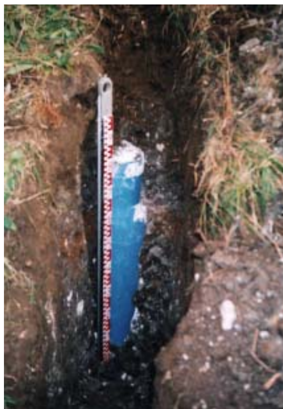
(a) Lined lime pile
