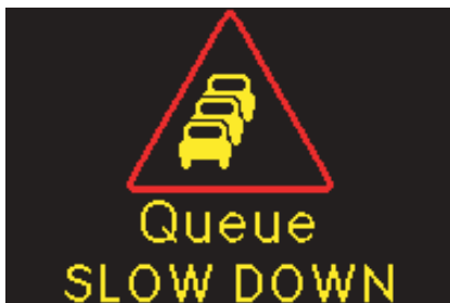
Figure 13 1500mm pictogram with one line of reinforcing text and one line of supplementary text
