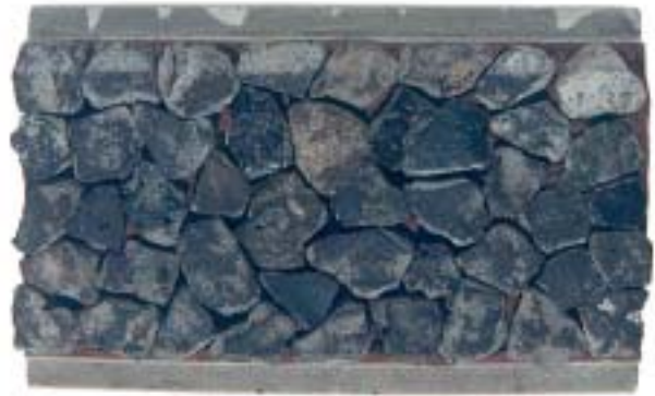
Figure 3.4 PSV specimen – (Laboratory B, reported PSV=53)
