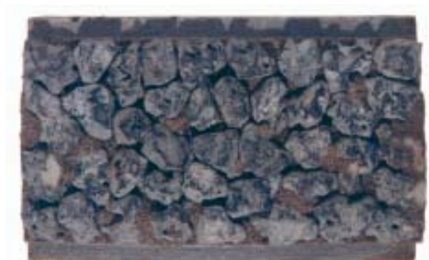
Figure 3.3 PSV specimen – BOS ‘random’ particles (TRL, reported PSV=56)
