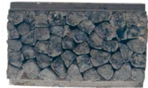
Figure 3.2 PSV specimen – BOS ‘regular’ particles (TRL, reported PSV=50)
