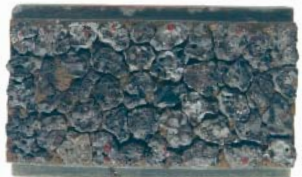
Figure 3.5 PSV specimen – (Laboratory D, reported PSV=58)
