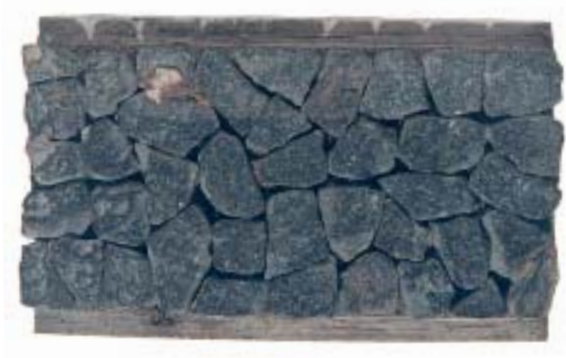
Figure 3.1 PSV specimen – control stone (TRL)
