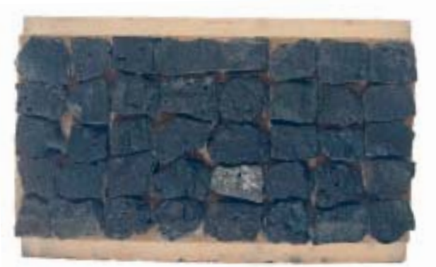
Figure 3.6 PSV specimen – (Laboratory A, reported PSV=65)
