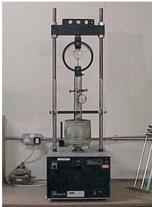
**Figure A6** Laboratory CBR test in progress
