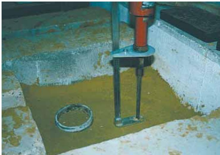
**Figure A5** Arrangement of DCP test
