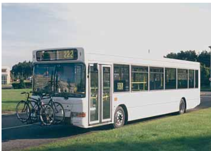
Plate A.1 The test bus fitted with the rack and two bicycles
