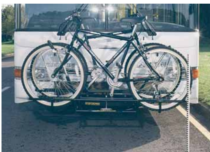
Plate A.2 Two bicycles in the rack, showing their positions in relation to the bus headlamps
