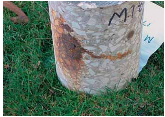
Figure 4.6 Examples of corrosion cracking
